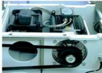
Maintenance-free servo drives with digital control
