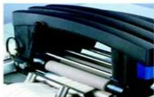
Automatic, self-adjusting lap monitoring is integrated in the top roll support
