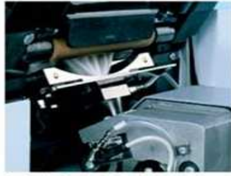
Pneumatic sliver threading device
