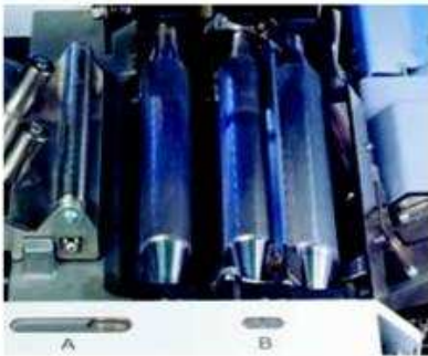
Precise quick adjustment of bottom cylinder distances
