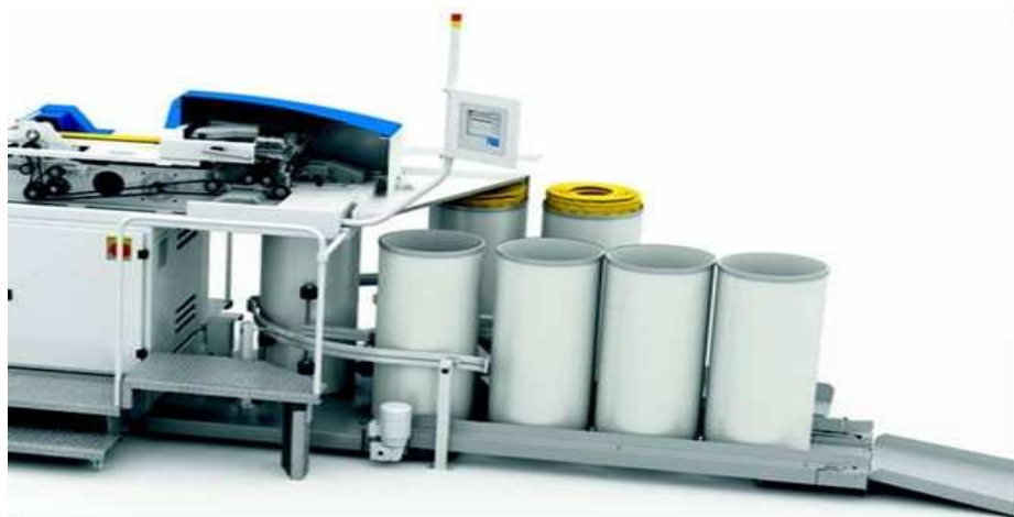
Automatic, self-adjusting lap monitoring is integrated in the top roll support
