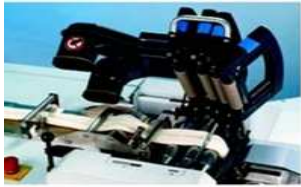
The drafting system can be opened with one single action. The top rolls remain safely in the top roll supports
