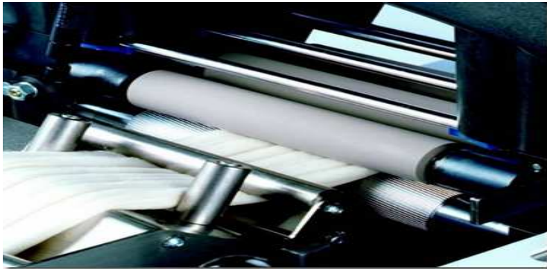
The drafting system can be opened with one single action. The top rolls remain safely in the top roll supports
