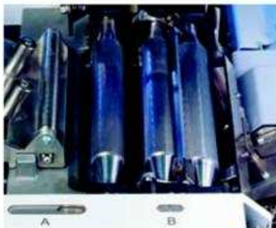
Precise quick adjustment of bottom cylinder distances
