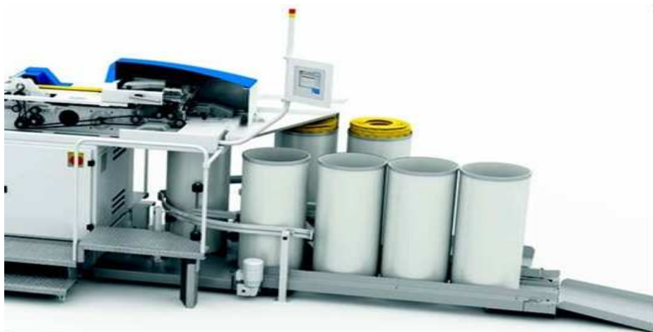
Automatic, self-adjusting lap monitoring is integrated in the top roll support
