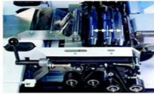
The drafting system is equipped with a quick adjustment unit. The drafting zone width can be directly read from two dials (A = break draft zone; B = main draft zone)
