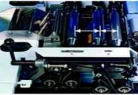
The drafting system is equipped with a quick adjustment unit. The drafting zone width can be directly read from two dials (A = break draft zone; B = main draft zone)
