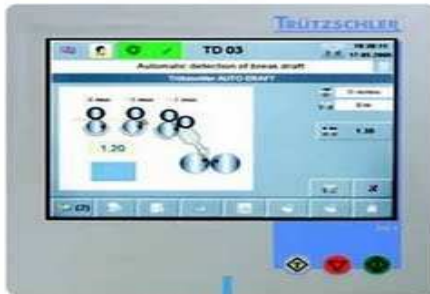
Start of the automatic break draft determination
