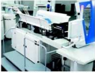
The hoods and the drafting system can be opened without tools within a few moments
