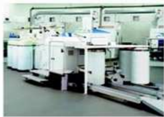
Autonomous can changer without mechanical connection to the draw frame
